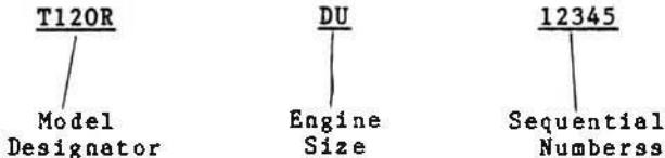
Engine Number - Located on left side of engine crankcase at base of cylinder. From 1968 the engine number is stamped on a raised boss in this location. Beginning in 1969 the boss was inscribed with the Triumph logo prior to the number being stamped. Beginning in 1965 the frame and engine numbers are the same (although some exceptions have been noted). Prior to 1965 these numbers were different.
